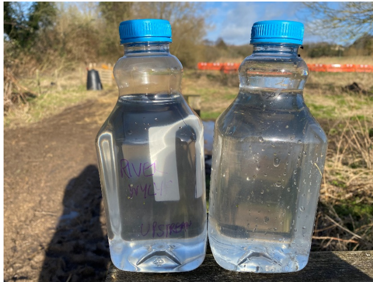
Photo 1: Samples taken on 17/02/22 when overflow was in operation: River Wylfe river water upstream of the reedbed on the left and influent to the reedbed on the right.
