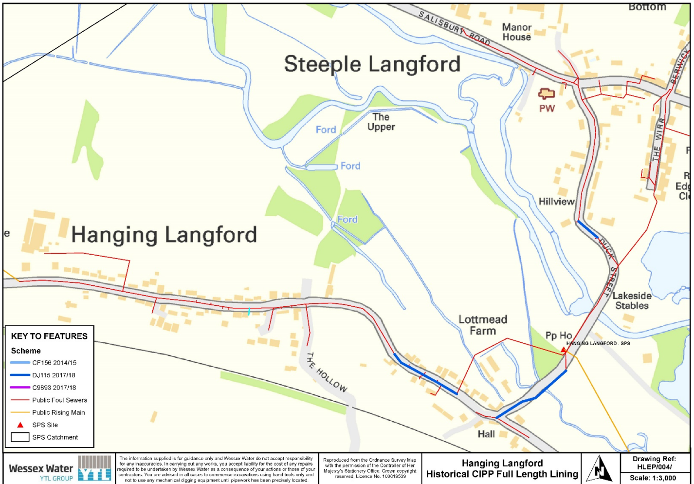
Plan 4. Sewers in Hanging Langford sealed since 2015 using cured in place pipe (CIPP) lining. DP0132 not shown.
